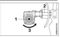
The axle (1) must be below the shaft (2).
