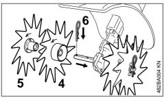
Rotate the inner right-hand blade (4) on the axle until it can be pushed into position – check the direction of rotation again (arrows).
